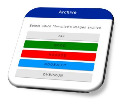
The new release is also improving the archive of the film-strip images, handling all the types of different classes independently
