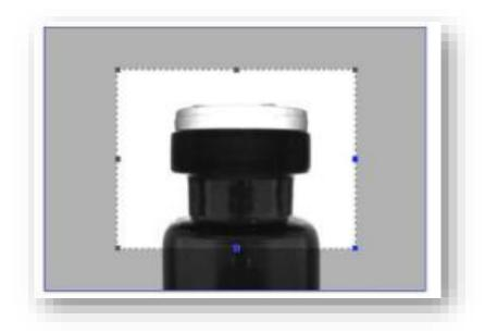
The ROI size can be set by using the mouse directly on the GUI or by sliders on the ROI parameter window or by editing the parameter value
